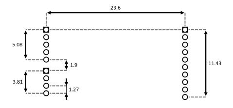
Figure 6. Drive PCB mating connections
