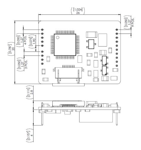
Figure 4. Drive PCB Geometry. Dimensions in mm [inches]
