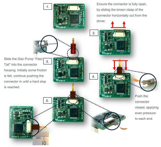
Visually inspect the connection, ~5mm should be exposed which would verify that the "Flexi Tail" is properly seated into the connector.
