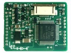
Figure 2. The General Purpose Disc Pump Drive PCB
