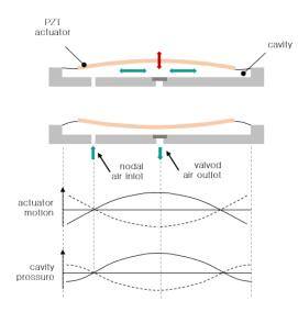
Figure 1. A schematic of the disc pump
