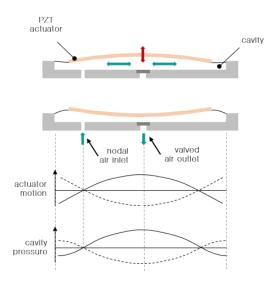
Figure 1. Principle of operation
