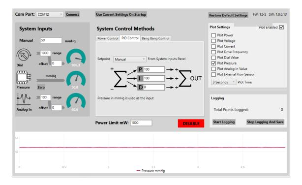
Figure 15. Pressure controlled to 50 mmHg under PID control mode
