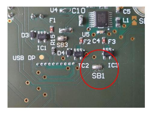
Figure 12. Solder applied to solder bridge "SB1" to enable power over USB
