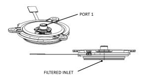
Figure 10. US Series pumps - port numbering
