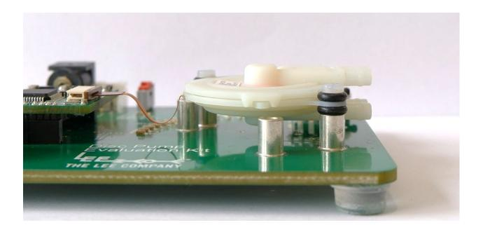
Figure 7. Example of recommend pump mounting
