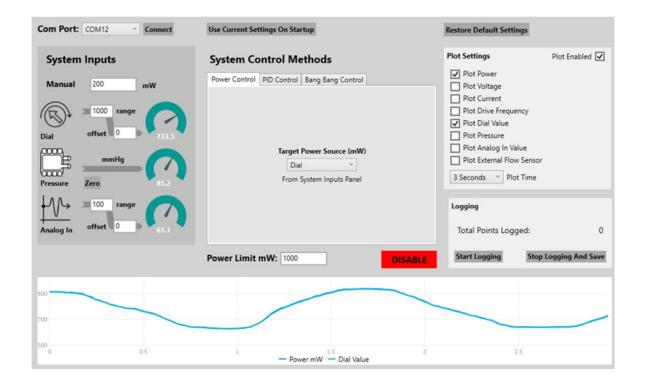
Figure 14. Power controlled to a target controlled by the SETPOINT dial on the motherboard.
