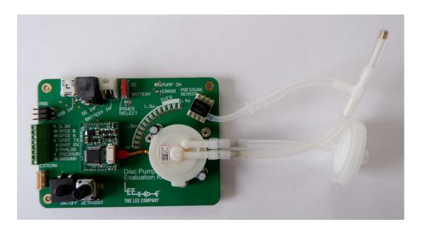
Figure 18. Pump setup tracking pressure via analog input
