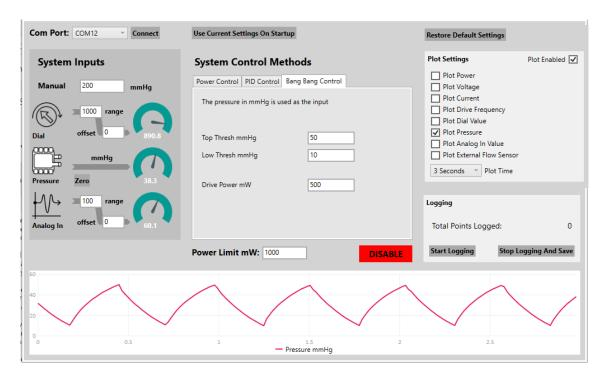
Figure 16. Pressure cycling between two limits under bang-bang control
