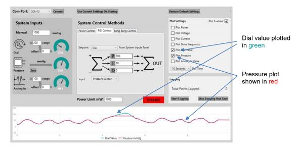
Figure 19. GUI showing PID control setup
