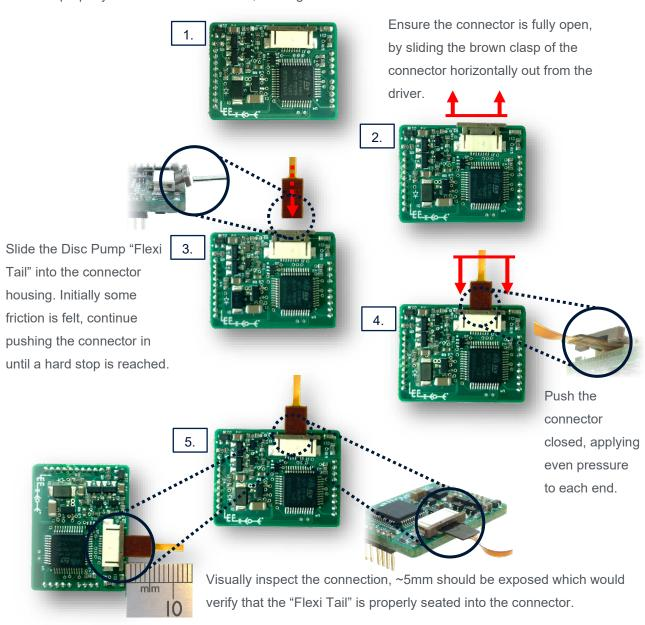
Figure 9. FPC connecting and reverse for removal
