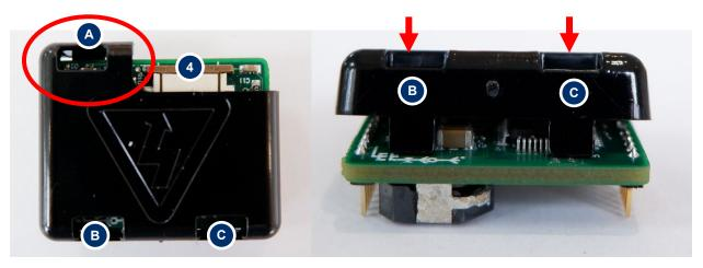
Figure 5. Fitting the protective cover to the General-Purpose Pump Drive PCB
