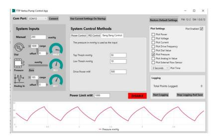
Figure 13. Disc Pump Control App GUI
