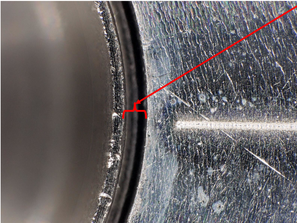
Photo 2: Plug placed in installation hole before installation process at 100x Magnification. Note the gap between the installation indicator feature on the plug and the installation hole (ref 0.2423 mm).
