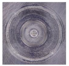
Photograph of a properly installed Betaplug which shows four staked tabs above the pin from the installation tool. The presence of these staked tabs and the pin being the correct distance below flush indicates a properly installed Betaplug.
