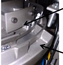
Separated pins and plugs fall off bowl track through use of a sorting plate and travel out of feed bowl.
