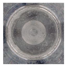
Photograph of a properly installed Betaplug which shows four staked tabs above the pin from the installation tool. The presence of these staked tabs and the pin being the correct distance below flush indicates a properly installed Betaplug.
