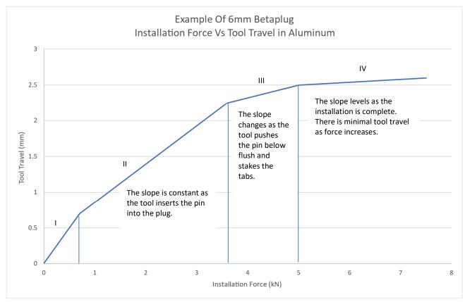
Using automated press equipment that monitors force and displacement has proven to be successful in ensuring consistent proper installation of the 6 mm Short Betaplug. The plot of Tool Travel vs. Install Force above illustrates the signature that defines the proper installation of a 6 mm Short Betaplug.
