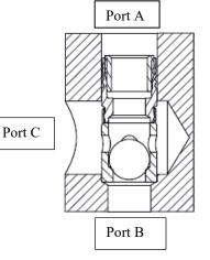
3. When the installation tool is retracted, the installed Shuttle Valve can be inspected by measuring the depth of the pin relative to the valve body. This distance should be flush to within 0.25 mm above flush. Port A is sealed by the expansion of the body outwardly into the hole and Port B is sealed by the nose of the valve seating into the bottom chamfered surface of the installation hole.
