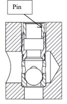
1. The Lee 5.5 mm Shuttle Valve is inserted into the installation hole with the pin end up as shown.
