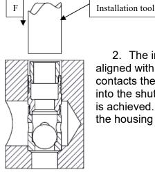
2. The installation tool (p/n CCRT0900120S) which is aligned with the installation hole, approaches the hole and contacts the back of the pre-installed pin. The tool drives the pin into the shuttle valve body until a force of 5338 to 6227 Newtons is achieved. Using friction and penetration, the lands bite into the housing material.
