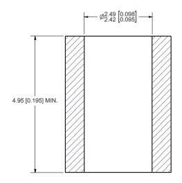
DIMENSIONS IN MILLIMETERS Note: Draft angle to fall within diameter tolerance Refer to Lee Drawing No. 1INST012735S
