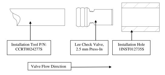
2. The installation tool (P/N: CCRT0024277S) is used to simply press the valve into a plastic installation hole until the valve is at a minimum flush with the top of the installation hole.
