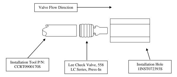
2. The installation tool (P/N: CCRT0900170S) is used to simply press the valve into a plastic installation hole until the valve is at a minimum flush with the top of the installation hole.
