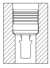
3. When the installation tool is retracted, the pin should be flush to within 0.25mm above flush of the insert body.
