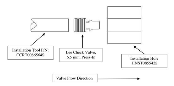
2. The installation tool (P/N: CCRT0086564S) is used to simply press the valve into a plastic installation hole until the valve is at a minimum flush with the top of the installation hole.
