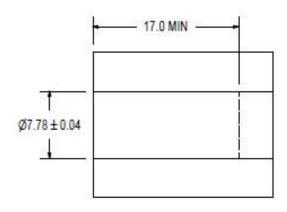
DIMENSIONS IN MILLIMETERS Note: Draft angle to fall within diameter tolerance Refer to Lee Drawing No. 1INST065550S
