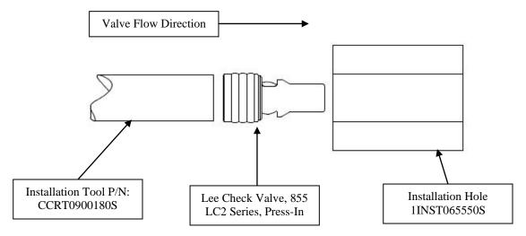
2. The installation tool (P/N: CCRT0900180S) is used to simply press the valve into a plastic installation hole until the valve is at a minimum flush with the top of the installation hole.
