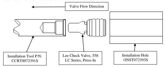
The installation tool (P/N: CCRT0072391S) is used to simply press the valve into a
