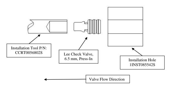
2. The installation tool (P/N: CCRT0056802S) is used to simply press the valve into a plastic installation hole until the valve is at a minimum flush with the top of the installation hole.
