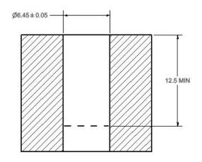
DIMENSIONS IN MILLIMETERS Note: Draft angle to fall within diameter tolerance. Refer to Lee Drawing No. 1INST085542S for complete specifications.
