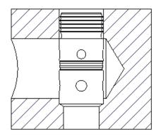
2. When the installation tool is retracted, the pin should be flush to within 0.25 mm above flush of the insert body.
