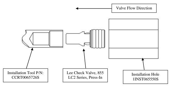
2. The installation tool (P/N: CCRT0065726S) is used to simply press the valve into a plastic installation hole until the valve is at a minimum flush with the top of the installation hole.
