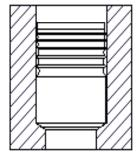
3. When the installation tool is retracted, the pin should be flush to within 0.25mm above flush of the insert body
