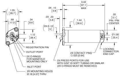
Unless otherwise specified, dimensions are in inches [mm]. Drawings are not to scale.
