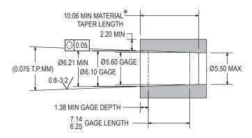
\* Depth of tapered hole from depth of 6.21 minimum diameter.
