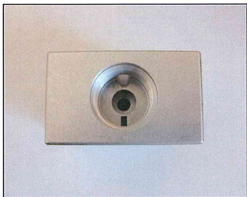
Installation hole is clean and free of debris.
