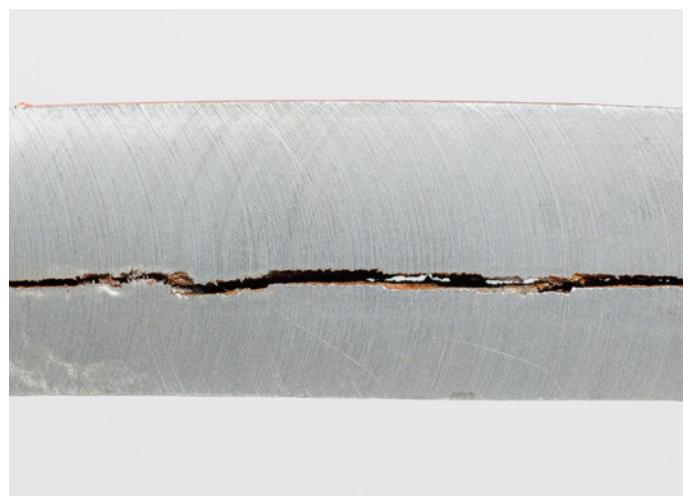
Example of cracking caused by hydrogen embrittlement
