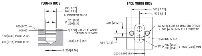
Boss geometries and dimensions shown above are for reference only. All dimensions are in inches [mm]. Reference Drawing Number LCFX0300250B for complete Plug-In Boss specifications and Drawing Number LFIX1002050A for complete Face Mount Boss specifications. Plug-In Boss geometry may be created using Lee cutting tool Part Number TTTA0000250B.
