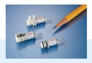
Wetted materials: housing (PBT), armature/core (FeCr Alloy), spring (316 SS), O-Ring (FKM) and epoxy. See table below for seal and plunger head wetted materials.
