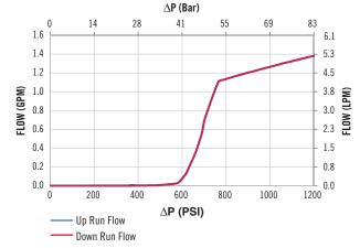
Typical Flow Curve for 40 Bar Valve
