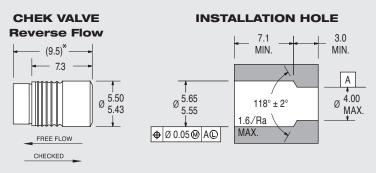
\*LOA before installation. All dimensions in millimeters, except where noted.
