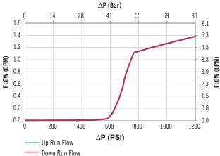
Typical Flow Curve for 40 Bar Valve
