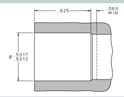
Forward burst direction – toward 45° seating shoulder Reverse burst direction – away from 45° seating shoulder
