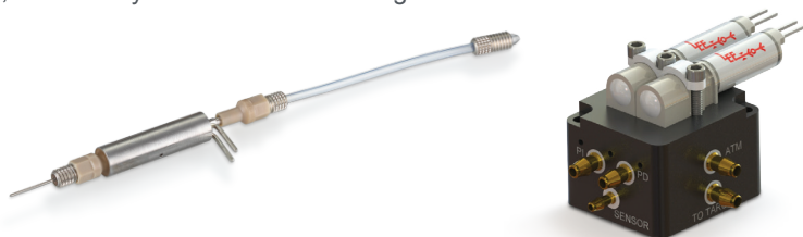
Left: A VHS Series dispense valve shown with an interchangeable threaded nozzle on the outlet and MINSTAC® fitting assembly threaded into the inlet. Right: The compact LFMX0534570B Reversible Flow Manifold (29 x 25 x 19 mm) comes with two LHD Series valves and is plumbed to enable switching between vacuum and pressure.
