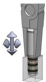
Figure 5: Install valve retention bracket if the valve's NC port is to be subjected to 15 PSIG or greater.
