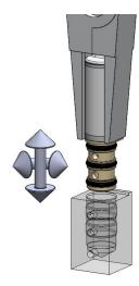
Figure 4: Load until the alignment flange mates to the manifold.
