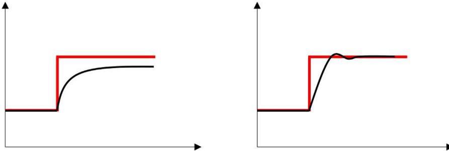
Figure 6 Step input (0<sup>th</sup> degree) - Proportional control (P) steady state error (left) and Integral (I) control no steady state error (right)
