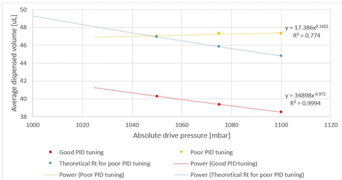
Figure 5 Dispensed volume vs Drive pressure for different PID tuning
