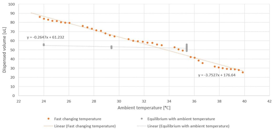
Figure 8 Dispersed volume vs temperature for different temperature-time gradients.
