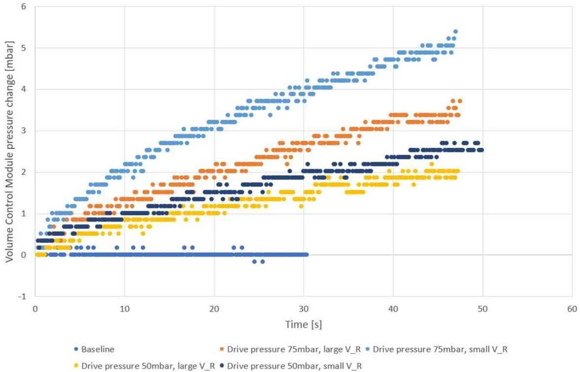
Figure 12 Changes in the pressure of the Volume Control Module due to self-heating. Data presented for various Fluid reservoir volumes and pressures (corresponds to different pump power).
