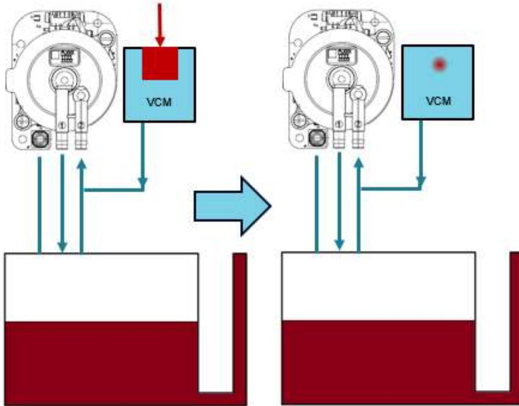
Figure 9 Warm air entering the system. As the air cools down, it creates a partial vacuum.
