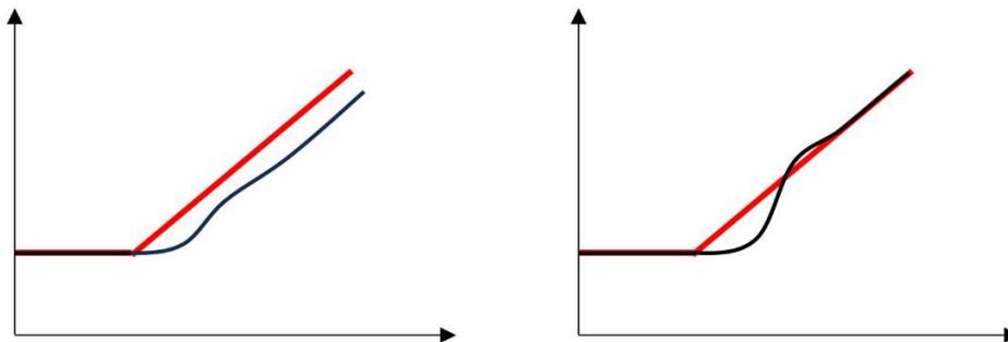
Figure 7 Ramp input (1<sup>st</sup> degree)– Integral (I) control steady state error (left) and Integral squared (I<sup>2</sup>) control no steady state error (right)
