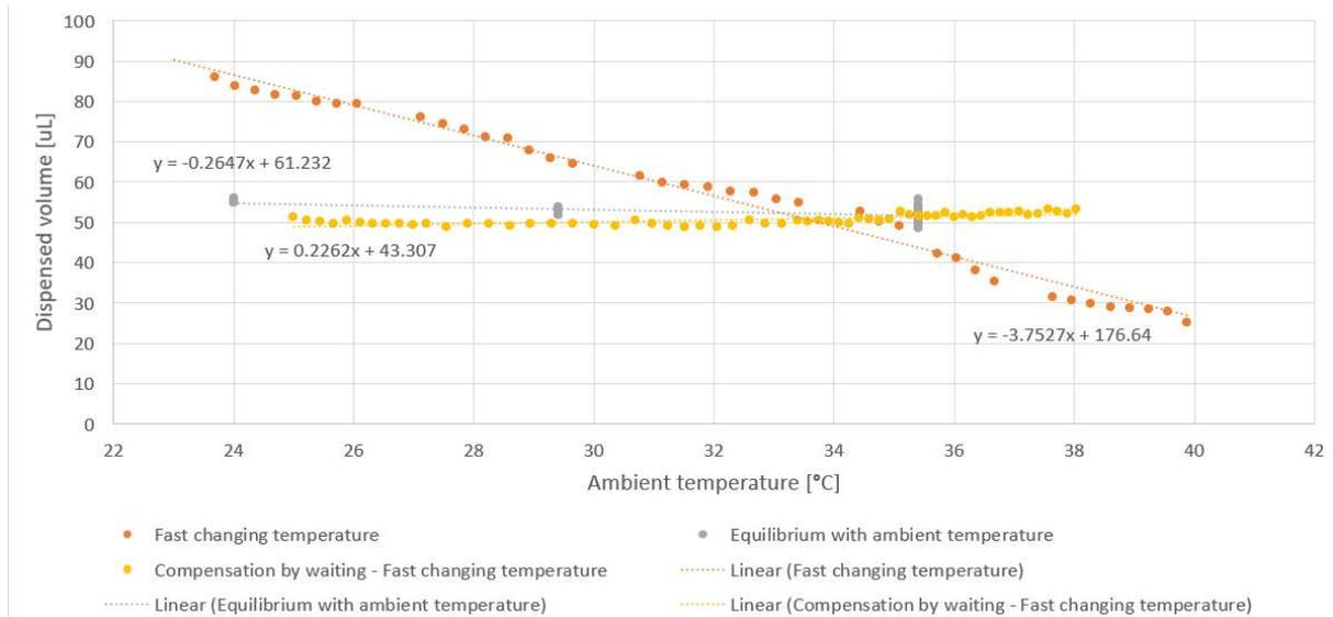
Figure 10 Dispensed volume vs temperature for different temperature-time gradients, with and without wait period upon air intake. Note that the data is noisy due to imprecise temperature measurements.
