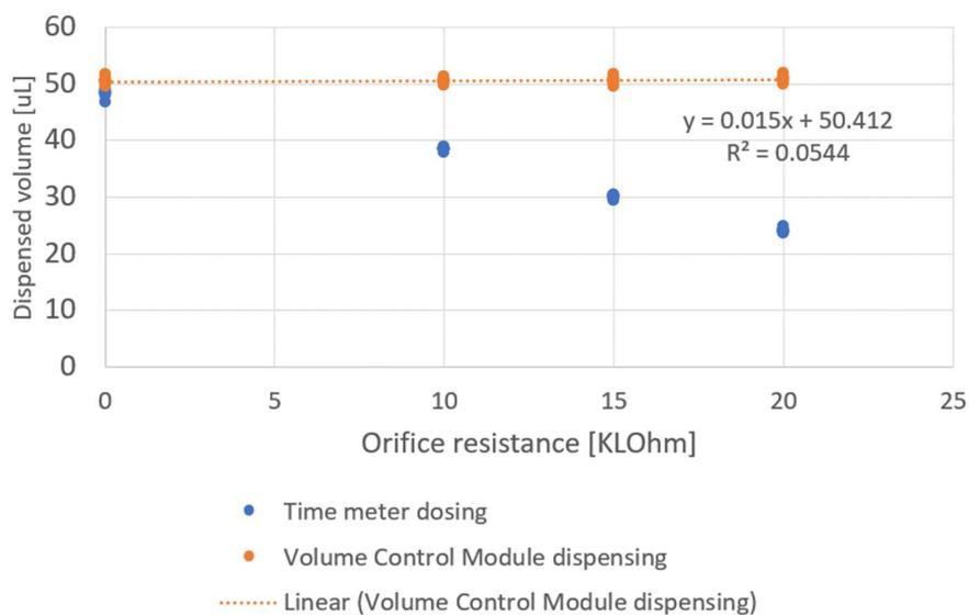
Figure 1 Liquid viscosity simulation – Volume Control Module dispensing vs Time-metered dosing
