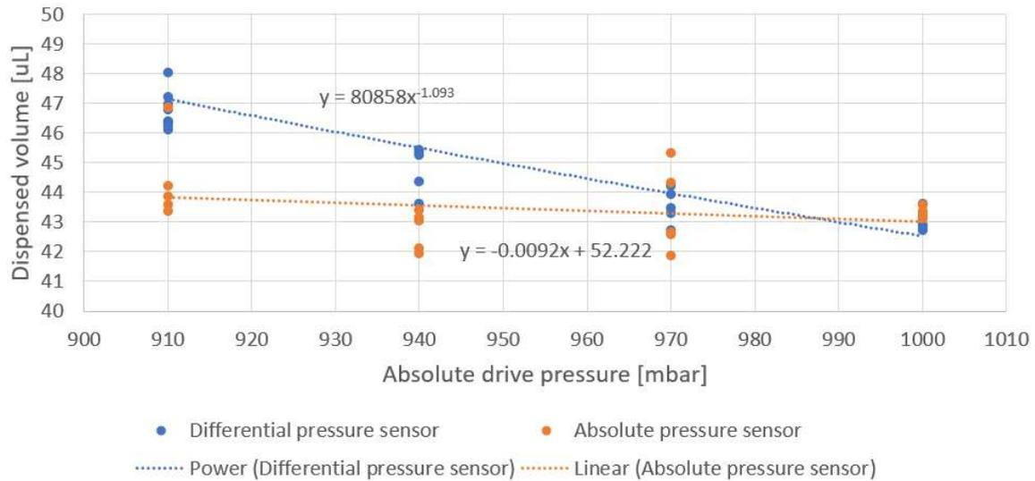
Figure 11 Dispersed volume vs ambient pressure for differential and absolute pressure sensor. The changes in atmospheric pressure were achieved using a vacuum chamber. Note that the data is noisy due to imprecise pressure control in the vacuum chamber.
