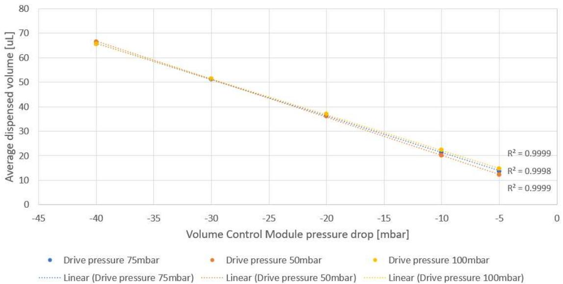
Figure 2 Dispersed volume vs VCM Pressure drop.
