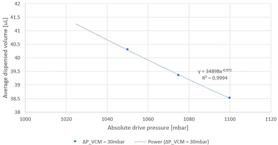
Figure 3 Dispensed Volume vs Drive pressure
