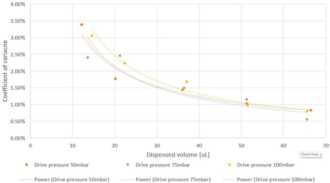
Figure 4 Coefficient of variation vs Dispensed volume
