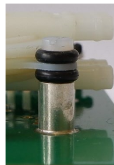
Figure 3. Example of mechanical pump mounting using two O-rings and a nylon box to prevent audible noise
