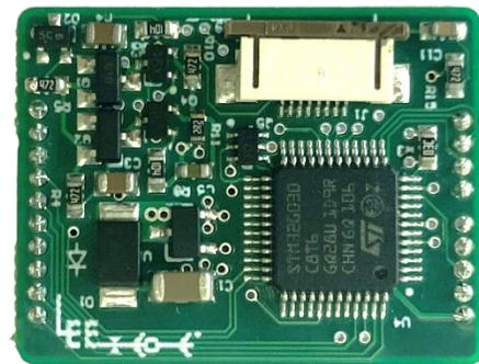
Figure 2. The General Purpose Disc Pump Drive PCB
