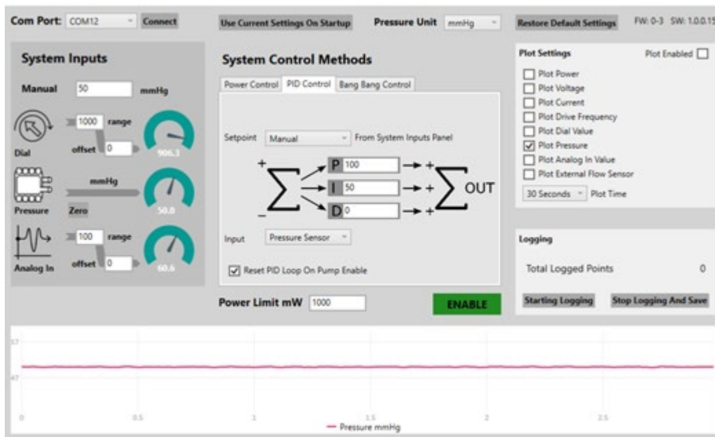
Figure 22. Pressure controlled to 50 mmHg under PID control mode
