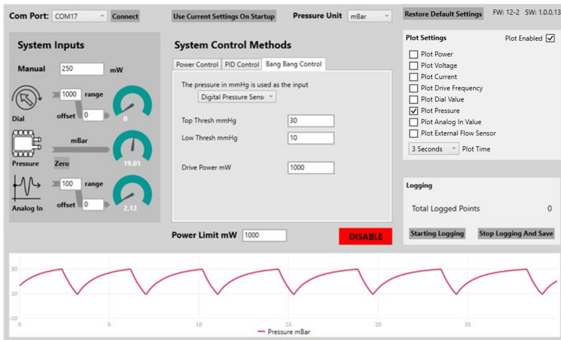
Figure 23: Pressure cycling between two limits under bang-bang control.
