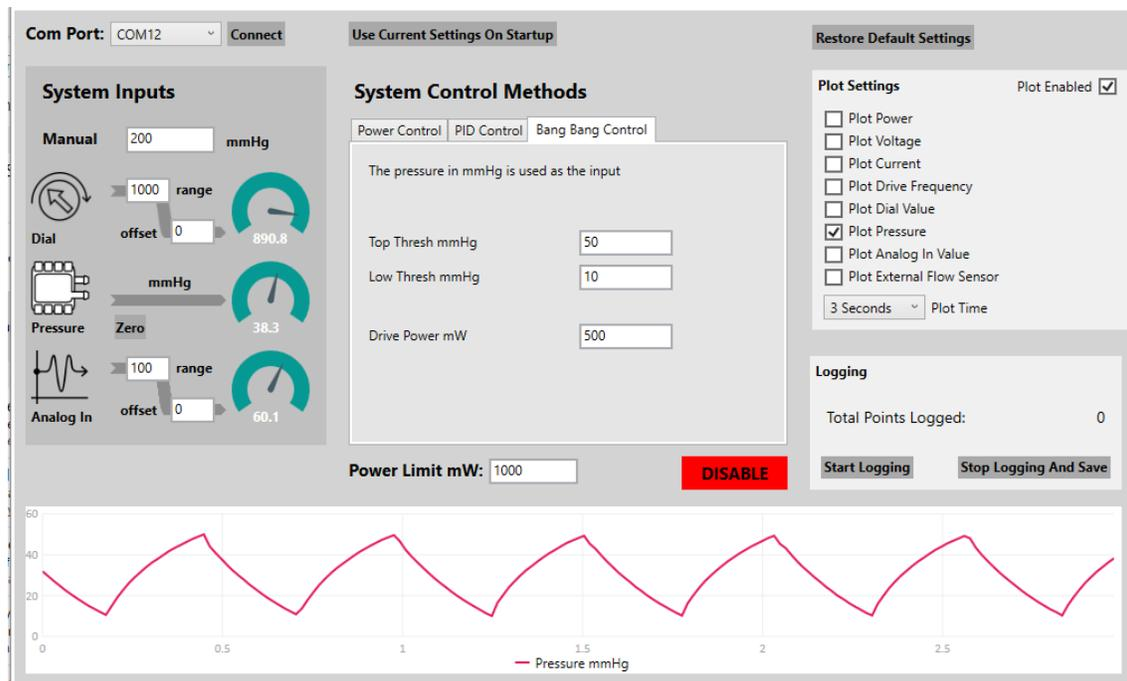
Figure 16. Pressure cycling between two limits under bang-bang control
