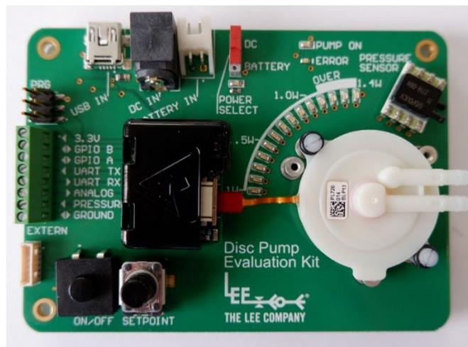
Figure 4. Disc Pump Evaluation Kit with the protective cover fitted to the General Purpose Disc Pump Drive PCB
