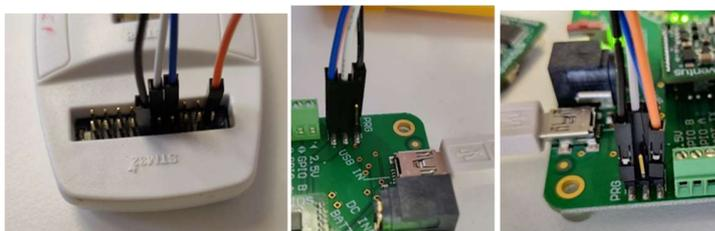
Note: The USB cable is used to deliver power to the Development Kit or Evaluation kit motherboards.
