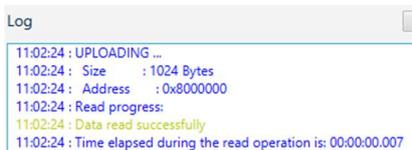
In the second tab navigate to the binary file (.bin) of the updated firmware. Set the start address to 0x08000000.
