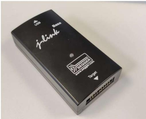
J-Link is a debug probe made by Segger (<https://www.segger.com/products/debug-probes/j-link/models/j-link-base/>).
