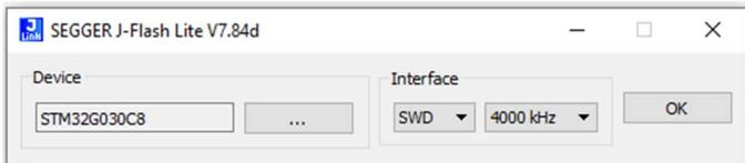
Once you have the programming screen opened, use the three dots to navigate to the binary file (.bin) of the updated firmware.
