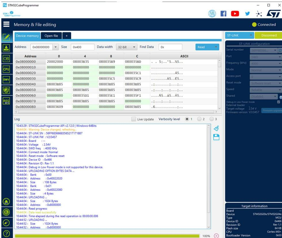
Click the Read button. This establishes the connection with the device. The log will confirm data being read from the device:
