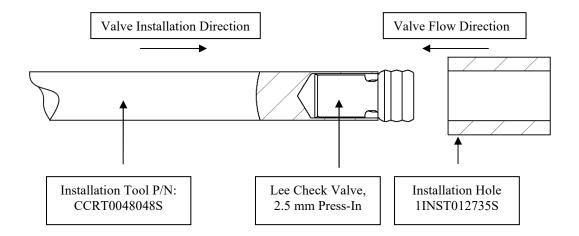
2. The installation tool (P/N: CCRT0048048S) is used to press the valve into the installation hole until the valve is, at a minimum, flush with the top of the installation hole.
