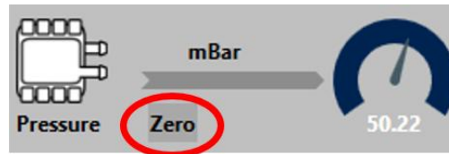
Figure 36. Zeroing the pressure sensor
