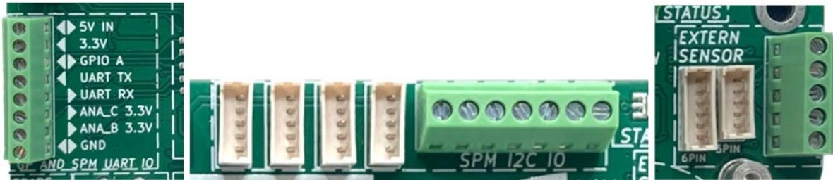
Figure 37. Screw terminals for connecting analog sensors to the Development Kit. The sensor output can be connected to the GP driver or SPM UART IO (left) or SPM I2C IO (centre) and should be powered by the regulated voltage output of the EXTERN SENSOR connector (right). The pinout of the terminals can be checked on the back of the board.
