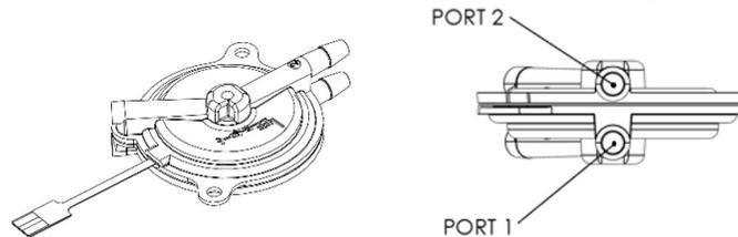
Figure 10. HP Series pump - port numbering.
