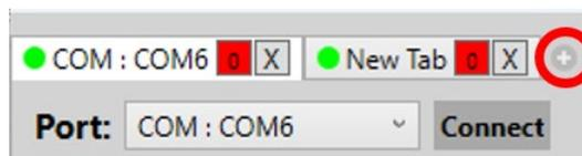
Figure 60. Adding and removing additional pump control tabs.
