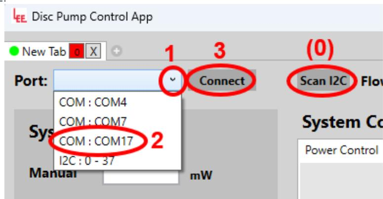
Figure 40 Connecting a driver board to the Disc Pump Control App
