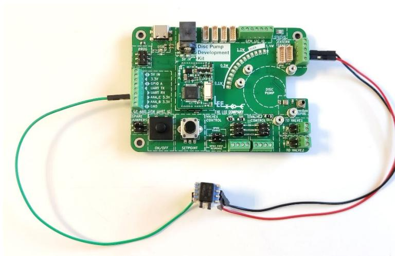
Figure 38. Analog pressure sensor connected to GP driver. Sensor is powered by the stable 3.3V for sensors.
