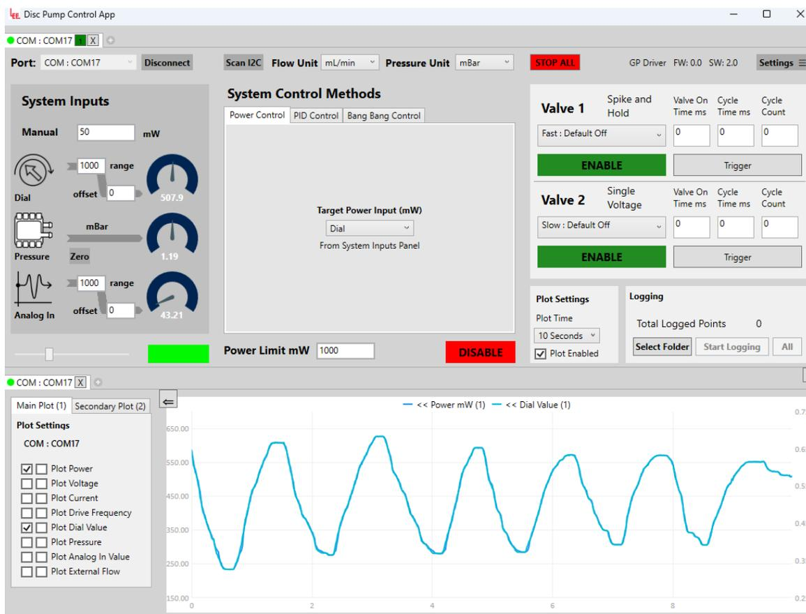
Figure 44. Power controlled to a target controlled by the SETPOINT dial on the motherboard.
