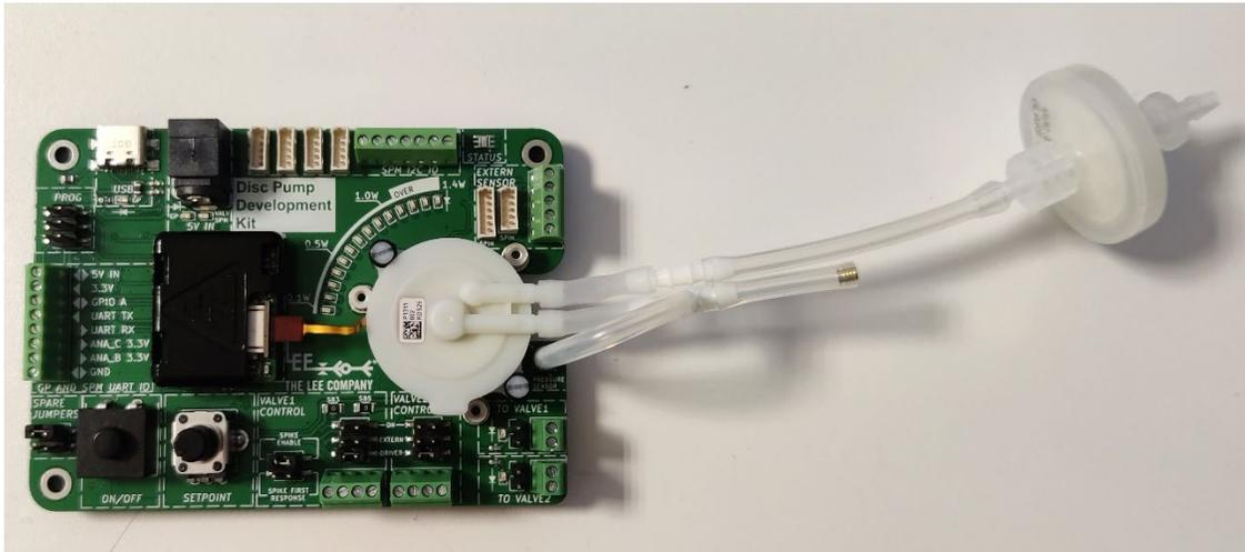
Figure 58. Pump setup tracking pressure via analog input
