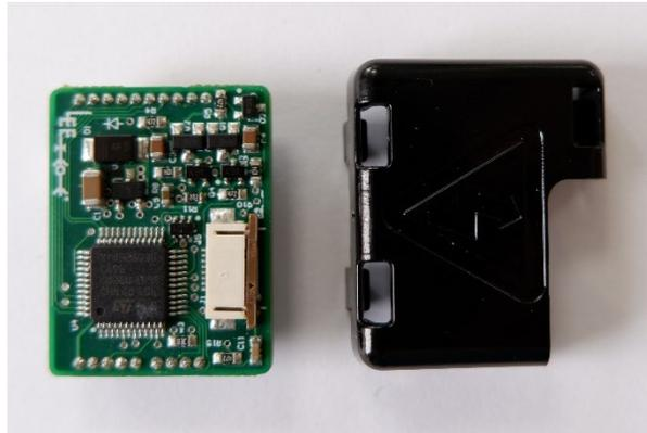
Figure 3. General Purpose Disc Pump Drive PCB (left) and protective cover (right)
