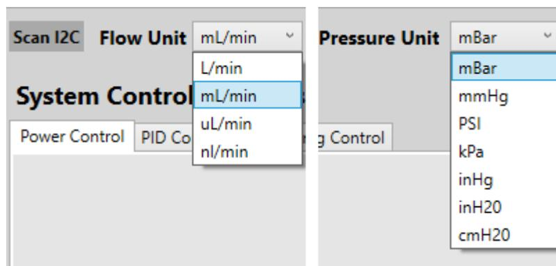
Figure 48. Selecting measurement units for flow and pressure.
