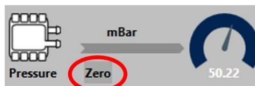
Figure 49. Zeroing the pressure sensor.
