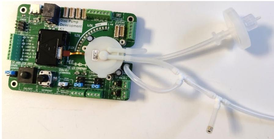
Figure 16. Disc pump output connected to the on-board pressure sensor and using a bleed orifice.
