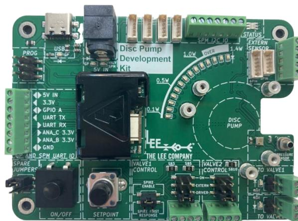
Figure 4. Disc Pump Development Kit with the protective cover fitted to the General Purpose Disc Pump Drive PCB
