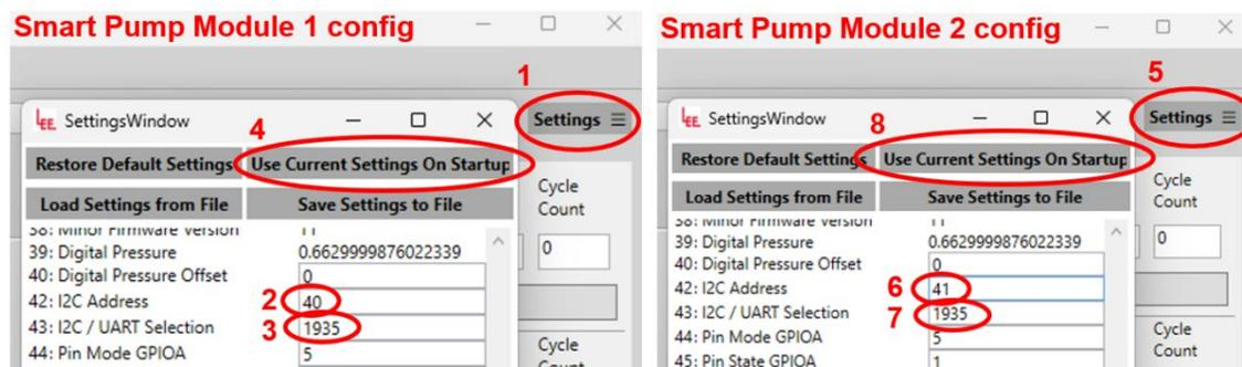
Figure 28. Configuring two Smart Pump Modules to be used at the same time over I2C. Note that Smart Pump Module needs to be restarted after acknowledging the Use Current Settings on Startup (step 4 and 8).
