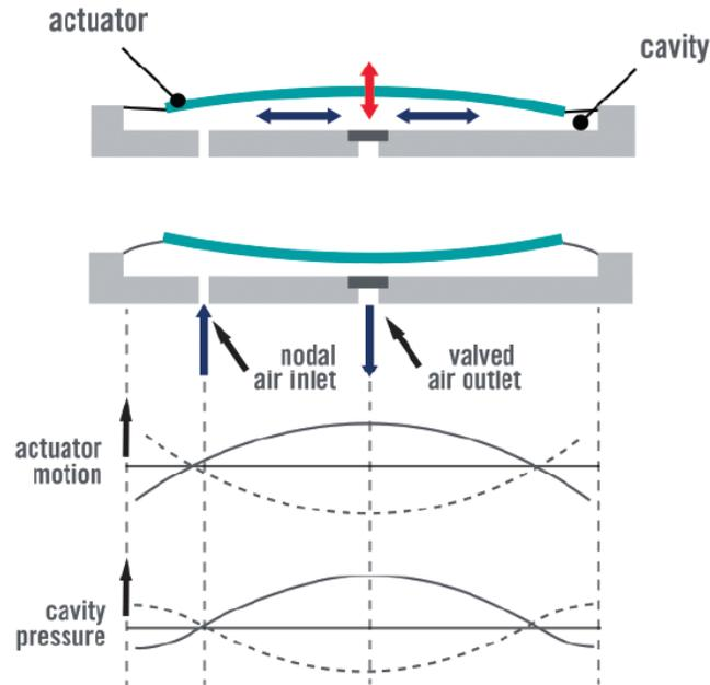
Figure 1. Principle of operation
