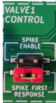
Figure 34. First response spike for VHS valves
