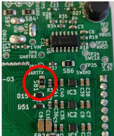
Figure 21. Remove "SB1" to disable power over USB
