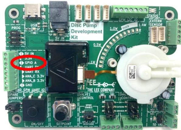
Figure 57. GPIO A is used for gating
