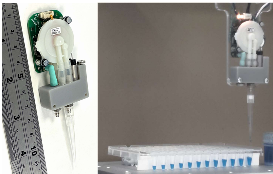
Figure 2: Left - Prototype VCM system, using The Lee Company Smart Pump Module and a custom pipetting manifold block. Right - Using the same prototype to dispense aliquots of increasing volume into successive wells of a 96-well plate.
