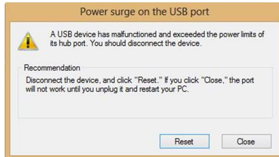
Figure 20. Error when connecting the Development Kit to a low power USB port
