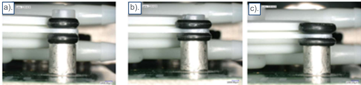
Figure 18. Images showing O-ring appearance as the nylon bolt is tightened. O-rings should be well compressed as shown in (b). Under tightening (a) or over tightening (c) may lead to audible noise
