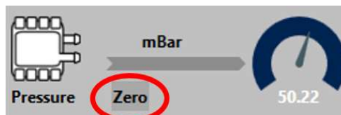
Figure 49 Zeroing the pressure sensor.
