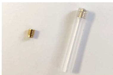
Figure 15 Orifice (left) and orifice installed in a tube (right).
