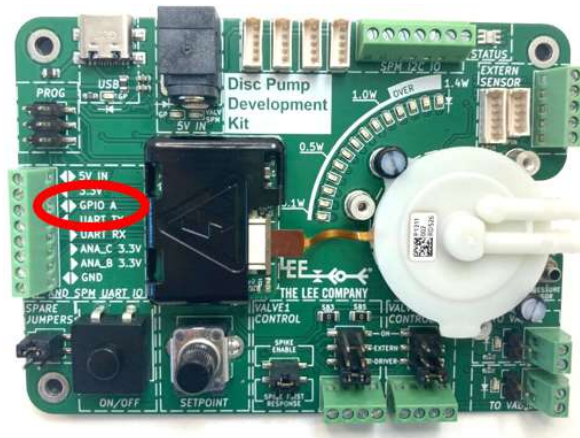
Figure 57. GPIO A is used for gating
