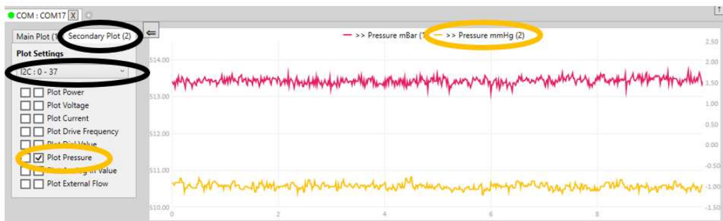
Figure 54 Plotting data from multiple pumps. Data from the main pump is plotted in red and data from the secondary pump is plotted in orange.
