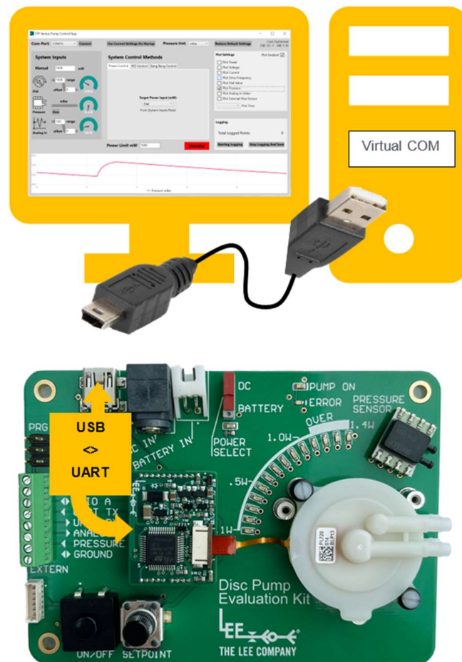
Figure 4 Connecting the Evaluation Kit Motherboard to a host PC.
